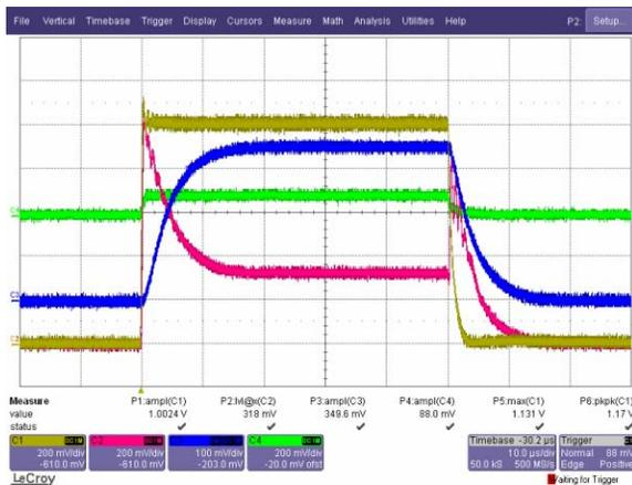
Figure 5: RF signals for RFQ
