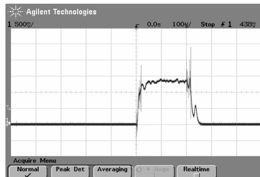
Figure 3: Beam signal at the LEBT exit
