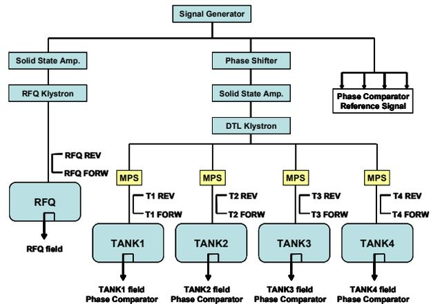
Figure 7: Schematic layout of the RF power flow
