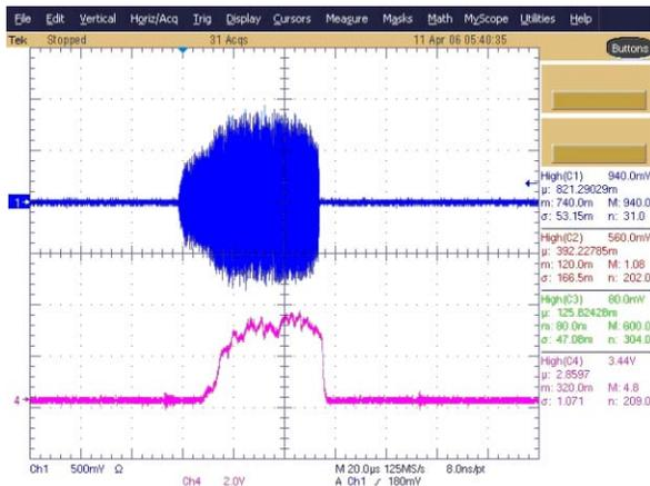
Figure 9: Beam Signals (CH1: ~1mA at RFQ exit, CH2: ~1mA at DTL exit)
