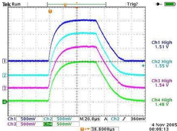
Figure 8: Cavity field waveform (CH1: tank1, CH2: tank2, CH3:tank3, CH4:tank4)
