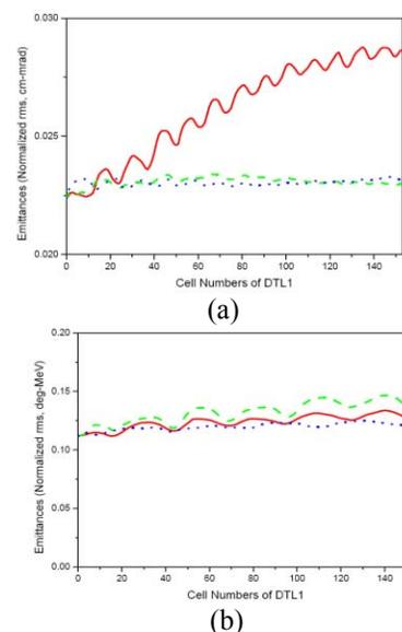
Figure 2. Transverse (a) and Longitudinal (b) emittances in DTL1: real (red), green (dashed), blue (dotted) lines for first, second, and third cases, respectively.
