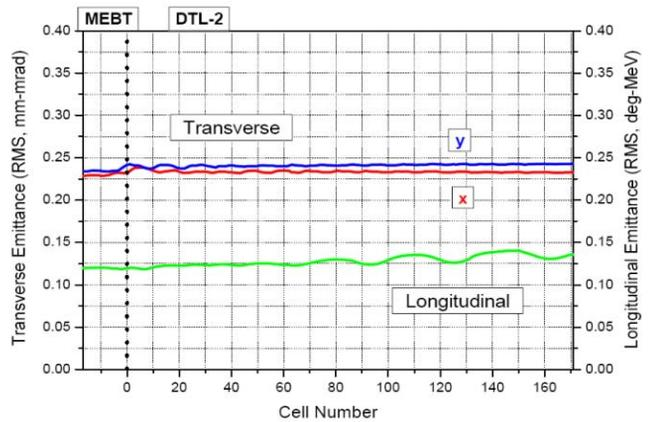
Figure 5. Transverse and longitudinal emittances without inter-tank matching.
