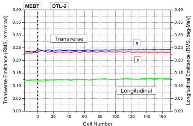
Figure 6. Transverse and longitudinal emittances with inter-tank matching.
