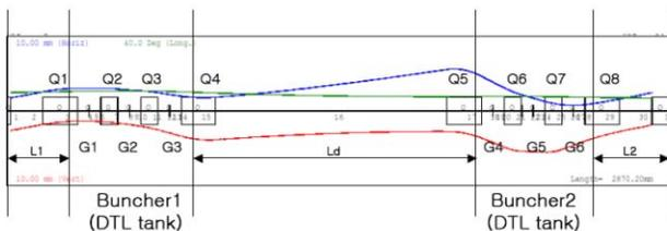
Figure 3. TRACE3D matching between DTL1 and DTL2.
