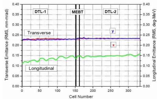
Figure 11. Transverse and longitudinal emittances.
