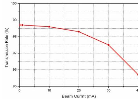
Figure 1. Transmission rates of the RFQ depending on beam currents.
