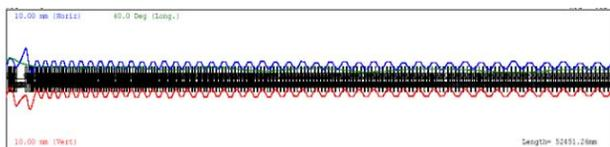
Figure 4. Beam simulation in the MEBT and DTL2: blue line in upper half plane, red line in lower half plane, green line between blue and green lines for horizontal (cm), vertical (cm), and longitudinal (degrees) beam sizes.
