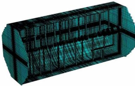
Figure 5: Schematic view of the cavity and PSS-4 accelerating structure.
