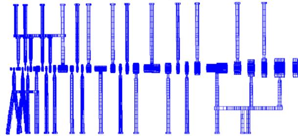
Figure 3: Schematic view of the PSS-4 accelerating structure.
