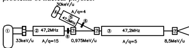
Figure 1: Scheme of the MILAC accelerator.
