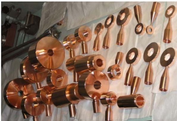
Figure 6: Photo of the drift tube cases.
