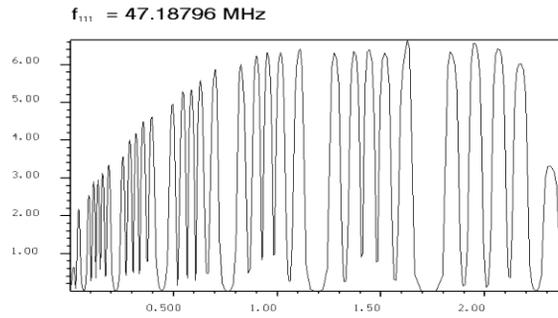
Figure 4: Distribution of the accelerating field along the gaps of the structure.
