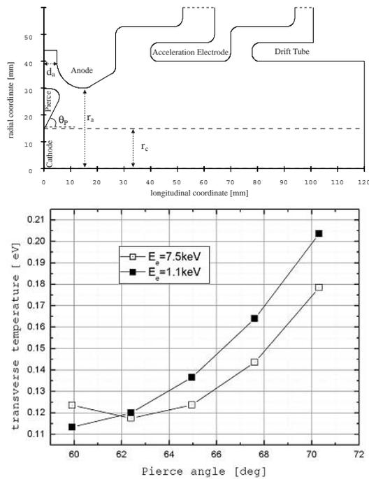
Figure 2: Up; schematic view of the electron gun, the cathode has a diameter of  $30 \text{ mm}$  and the Pierce electrode has an angle of  $\theta_P$ . Down; the transverse electron temperature is minimised for  $\theta_P = 62.9^\circ$ .
