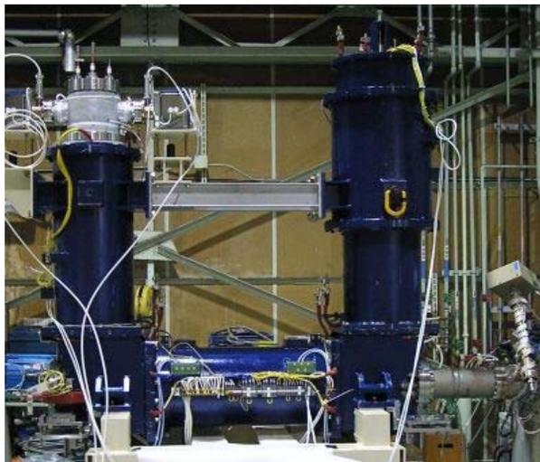
Figure 1: Picture of the constructed compact electron cooler. The cooling solenoid length is 0.8 m, the magnetic field 0.5 kG and the maximum expansion factor is 3.
