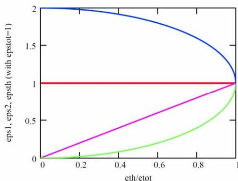
Figure 1: Flat beam emittances as function of  $\lambda$
