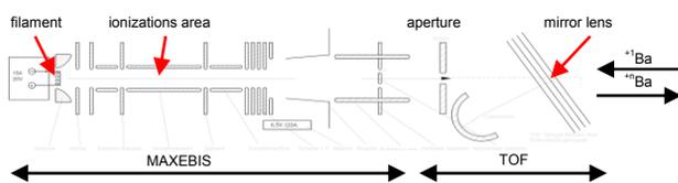
Figure 7: Inner structure of the MAXEBIS and the TOF spectrometer
