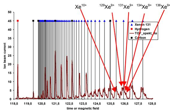
Figure 6: MAXEBIS TOF- Spectrum Xenon magnetic field 5T breeding time 25 ms, max.  $Xe^{11+}$
