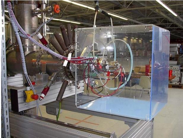
Figure 2: Electron gun of the MAXEBIS
