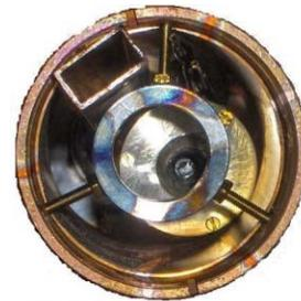
Figure 3: View (looking from plasma position) of the rf oven. Tube outer diameter 63 mm.
