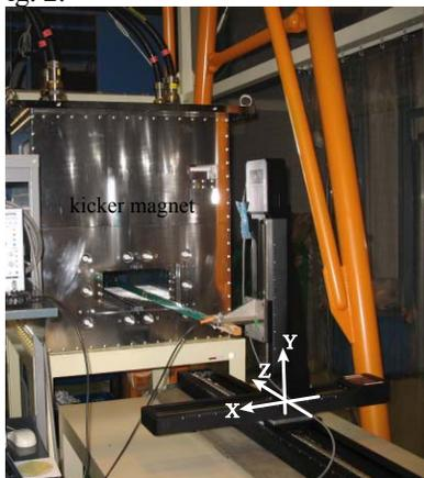
Figure 3: Setup of the magnetic field mapping. Definition of the direction of the 3 axes is also shown.
