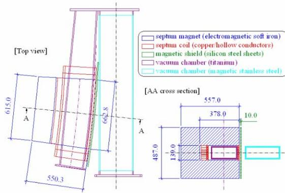
Figure 1: The schematic diagram of the injection septum 2 and the divergent duct in the injection line.
