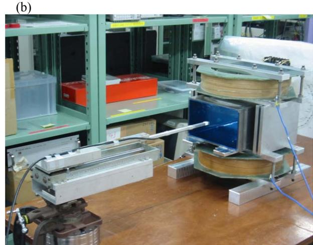
Figure 5: The field measurement set-up with the magnetic stainless steel duct.
