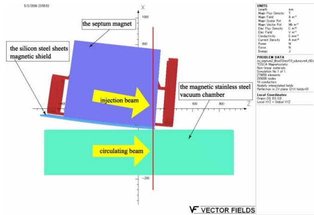
Figure 2: The typical 3D calculation model of the injection septum 2.
