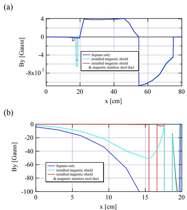
Figure 3: The result of the calculating field distribution along the intersect line with the circulating beam orbit perpendicularly in the position nearest to the septum magnet (refer the red line in the Fig.2).
