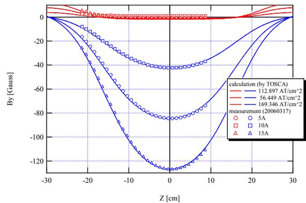
Figure 6: The results of the field measurement and 3D calculation. The blue lines show the field distributions produced by a Helmholtz coil without the test duct and the red lines shows the field distributions in the test duct.
