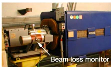
Figure 3: Beam loss monitor on a defocusing quadrupole.
