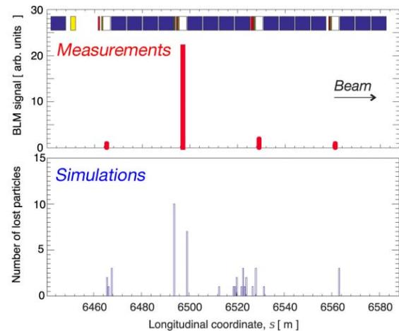
Figure 7: Measured (top) and simulated (bottom) losses at the SPS P6 ( $\approx 1.2$  km downstream of the collimator).
