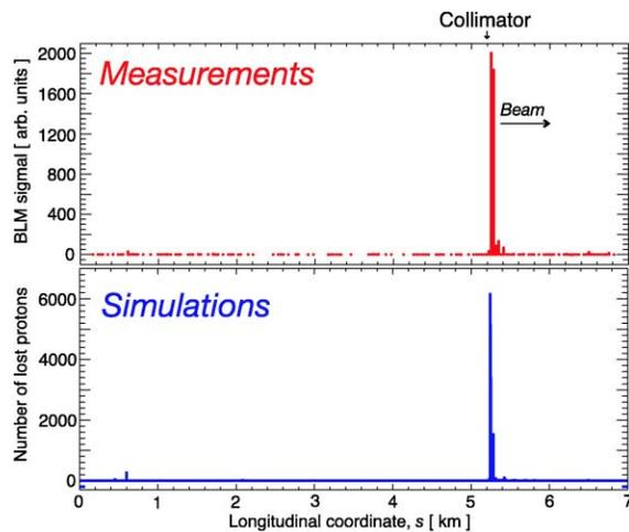
Figure 5: Measured (top) and simulated (bottom) beam losses around the whole SPS ring.
