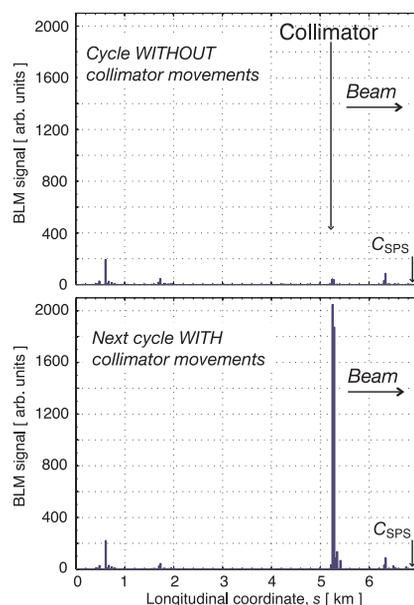
Figure 4: SPS loss patterns in consecutive cycles without (top) and with (bottom) jaw movements ( $C_{SPS} = 6911$  m).
