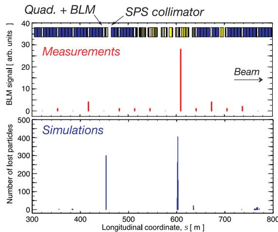
Figure 6: Measured (top) and simulated (bottom) losses at the SPS P2 ( $\approx 2.3$  km downstream of the collimator).
