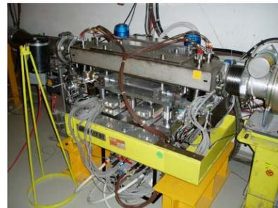
Figure 2: The LHC collimator prototype in the SPS tunnel.
