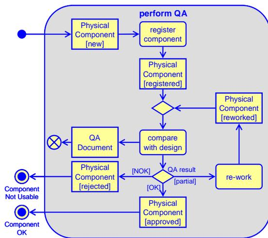
Figure 3: Process coordination using an Engineering Data Management System
