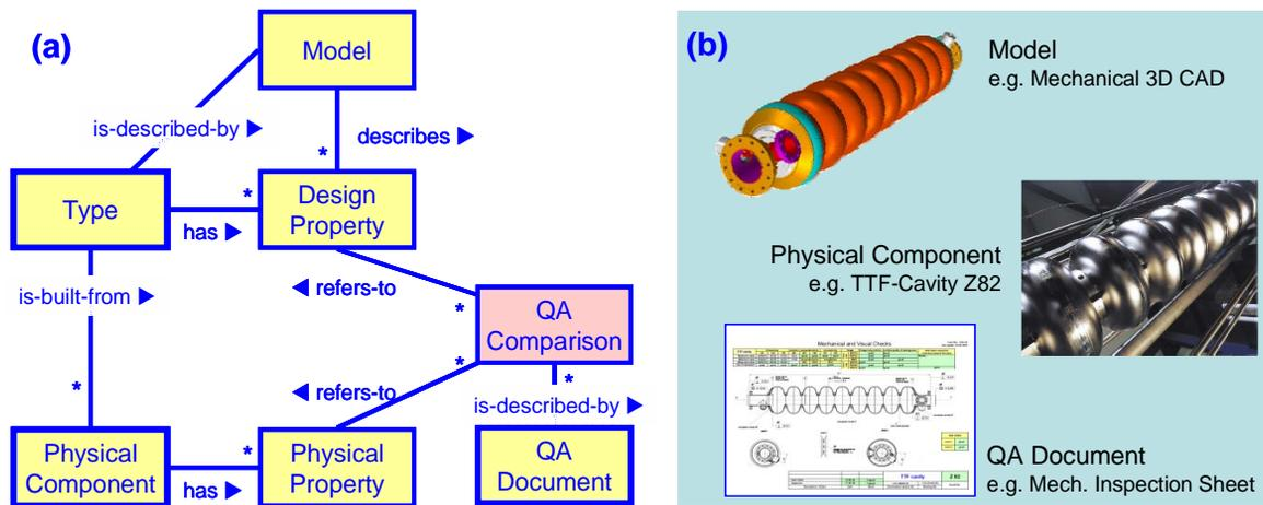
Figure 2: (a) Conceptual model for quality assurance (UML class diagram) and (b) examples.
