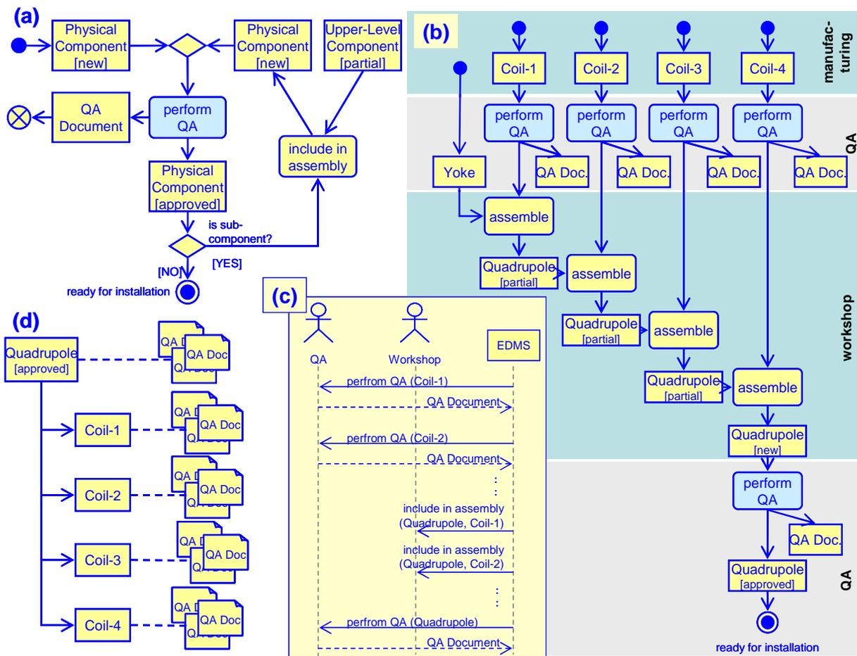
Figure 5: EDMS-based documentation of QA activities: (a) performing QA during manufacturing and assembly, (b) simplified example for quadrupole assembly, (c) EDMS coordinates process and records history, (d) final QA documentation objects in EDMS (Notation: UML).
