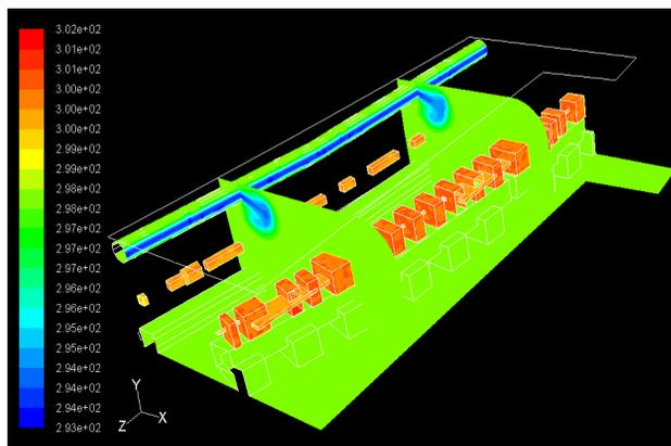
Figure 4: Simulated temperature field in the storage ring tunnel of the TPS.
