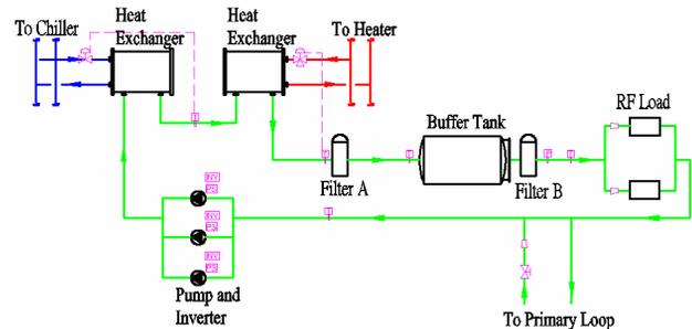
Figure 3: High precision water temperature control system.
