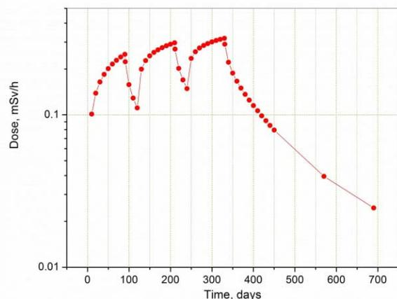
Figure 7: Calculated increase and decay of the accumulated dose rate in the vicinity of the slow extraction point of SIS100 synchrotron of FAIR.
