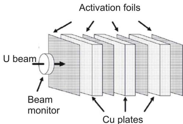
Figure 2: Target configuration
