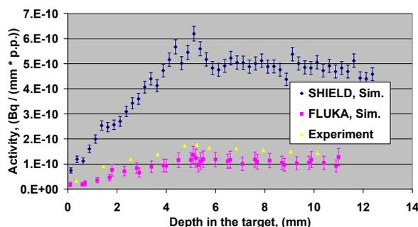
Figure 4: Activity of <sup>56</sup>Co: yellow – measured, lilac – FLUKA, blue – SHIELD.
