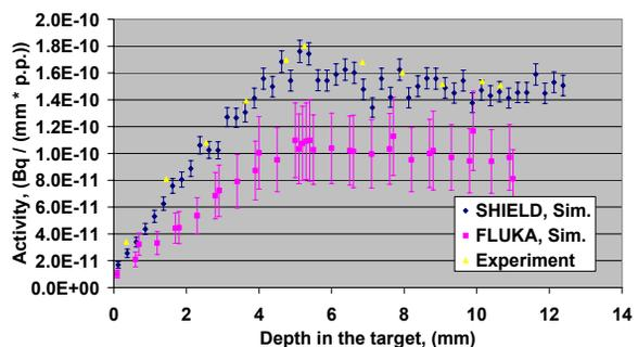
Figure 5: Activity of <sup>57</sup>Co: yellow – measured, lilac – FLUKA, blue – SHIELD.
