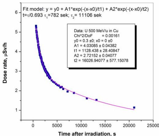
Figure 3: Decay curve for Cu target with 11 mm thickness irradiated by a <sup>238</sup>U beam with energy of 500 MeV/u for 20 h (total dose 4.66\*10<sup>11</sup> ions).
