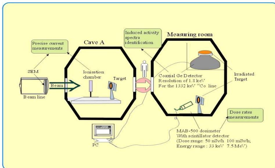
Figure 1: Experimental setup for the induced radioactivity measurements.
