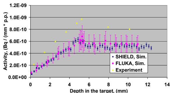
Figure 6: Activity of <sup>58</sup>Co: yellow – measured, lilac – FLUKA, blue – SHIELD
