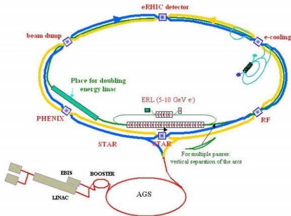
Figure 5: Layout of the RHIC accelerator complex with EBIS, electron cooling, and an ERL for eRHIC.
