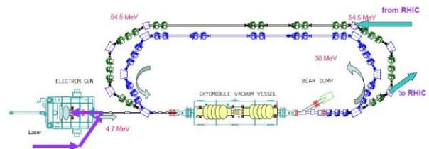
Figure 7: ERL layout with 2 turns for electron cooling of RHIC beams [22].
