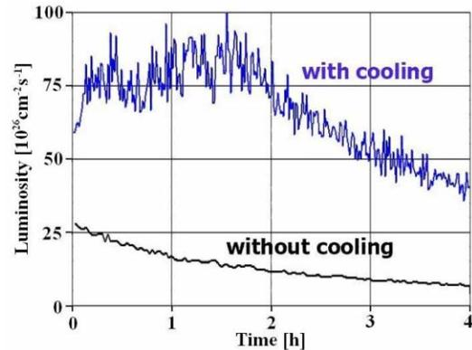
Figure 6: Simulation of the Au-Au luminosity evolution with and without cooled beams [21].
