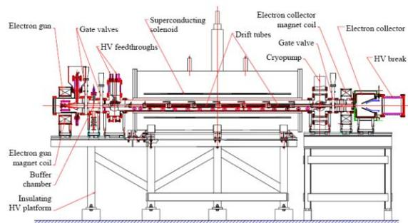
Figure 4: Schematic of the proposed EBIS for RHIC.
