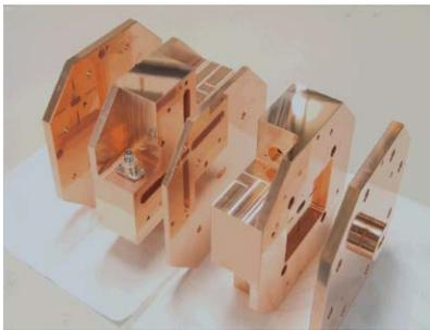
Figure 4: Cold model of IP-BPM system.
