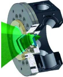
Figure 5: An Image of Laser Wire Chamber at ATF.
