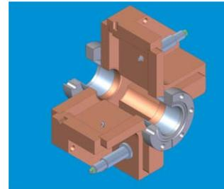
Figure 2: Cavity BPM with Slot Coupled Waveguide.
