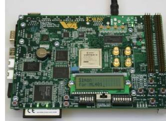
Figure 6: FPGA Board developed for FONT4.
