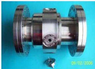
Figure 1: BPM Cavity and one of its feedthrough.
