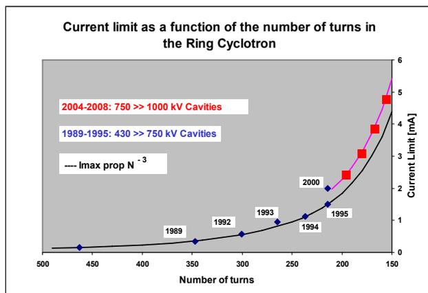
Figure 2: Observed and extrapolated current limit as a function of the number of turns in the Ring Cyclotron. The step between 1995 and 2000 is due to the improvement of the beam quality from the injector cyclotron.
