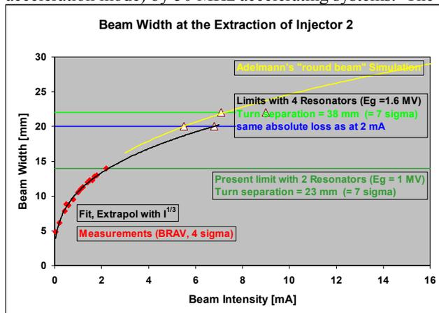
Figure 2: Expected beam width at the extraction of the injector cyclotron. The yellow line is the result of a full 3-D simulation.
