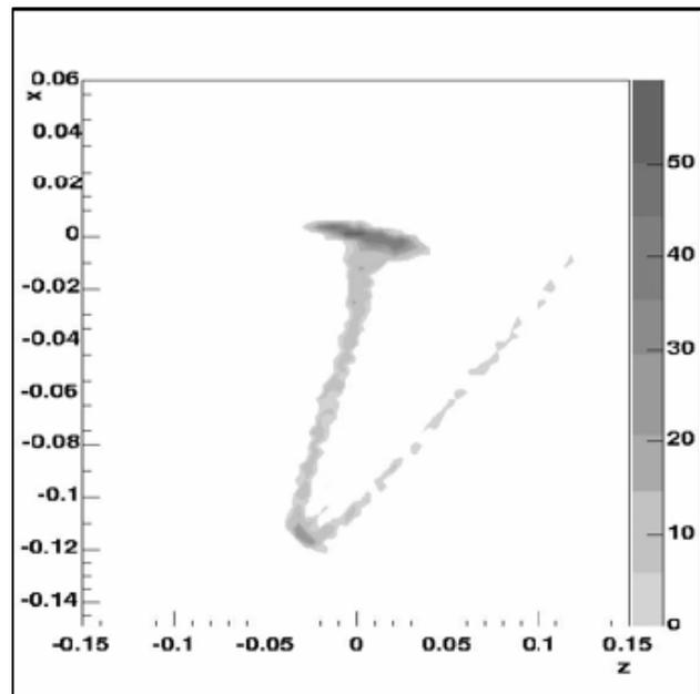
Figure 1: Density distribution of the beam entering the injector cyclotron after passing the first phase collimators.
