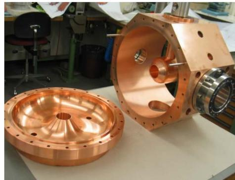
Figure 3: Double-gap drift tube buncher for the 72 MeV beam line.
