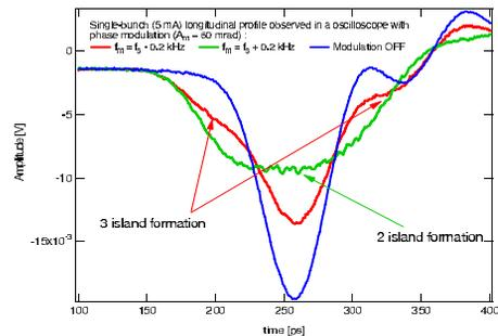
Figure 3: Beam profile observed in an oscilloscope.
