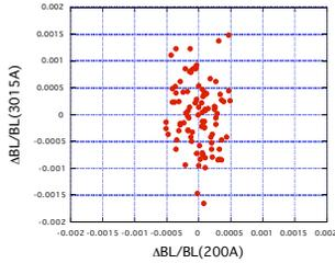
Figure 4: measured BL error of bending magnets.
