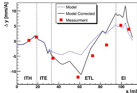
Figure 3:  $O^{4+}$  vertical trajectory measurements compared with the optics model prediction before and after the correction for the ITE bending dipoles quadrupole error.
