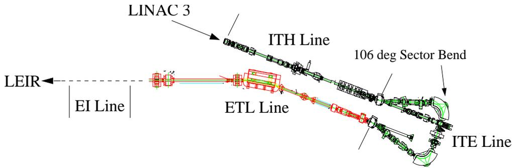
Figure 1: Transfer line drawing, the injection into LEIR is after the EI line.
