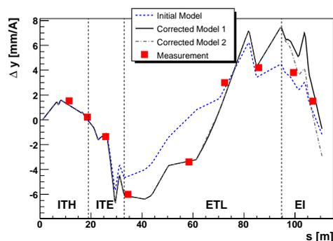
Figure 4:  $Pb^{54+}$  vertical trajectory measurements and comparison with the optics model prediction before and after the correction for the bending dipoles quadrupole error (see text for the difference between Model 1 and Model 2).
