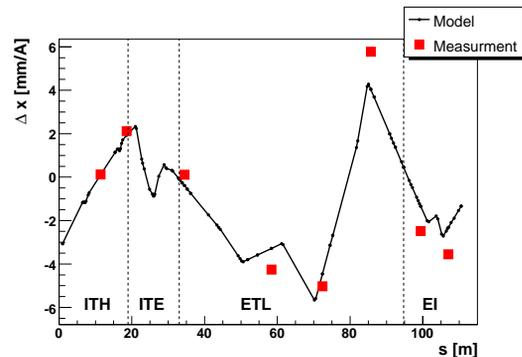
Figure 2:  $O^{4+}$  ions horizontal trajectory measurements and comparison with the optics model prediction.
