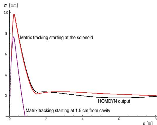
Figure 2: Comparison of reduced envelope calculations for the center slice.
