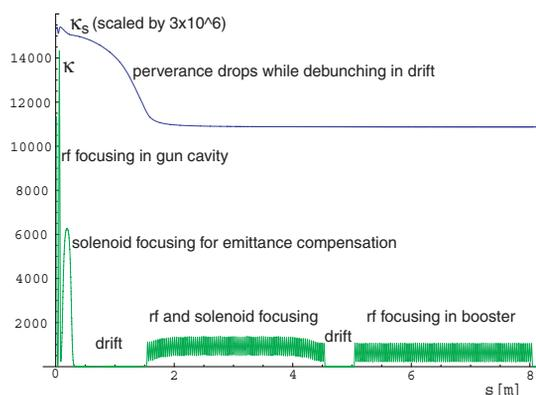
Figure 1: Focusing strength  $\kappa$  and perveance  $\kappa_s$  for the center slice. SPARC design courtesy of M. Ferrario.
