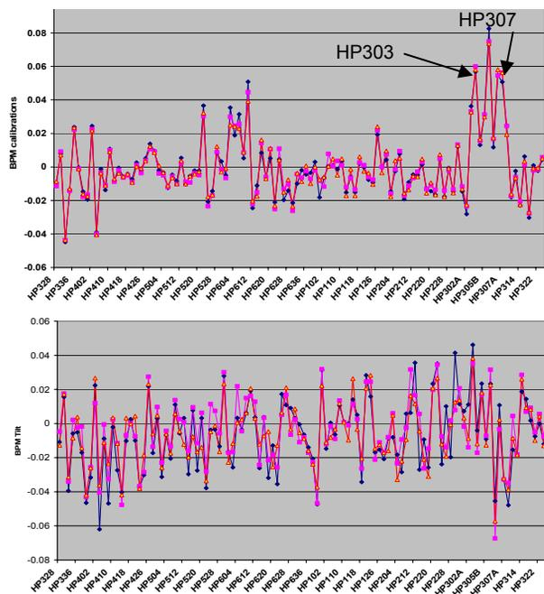
Figure 5: Top: Horizontal BPMs' gain errors; Bottom: Horizontal BPM Tilt
