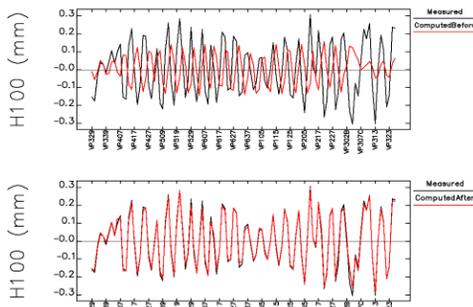
Figure 1: Typical measured and calculated vertical responses to a horizontal excitation before (Top) and after the fit (bottom).
