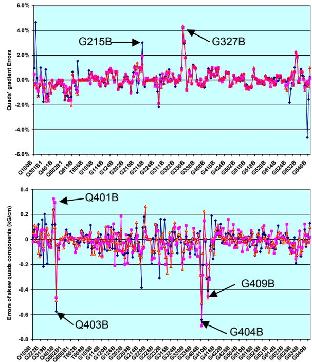
Figure 3: Top: quadrupole gradient errors; bottom: errors of integrated skew quads strength.
