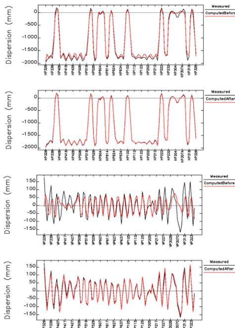
Figure 2: Measured and fitted dispersion in both horizontal (Top) and vertical planes (Bottom)
