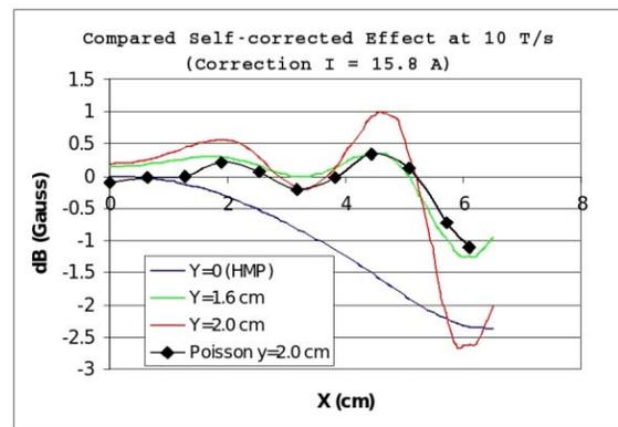
Figure 3: Field distortion for 10 T/s at 0, 1.6, and 2 cm above the HMP with the effect of the correction coils included.
