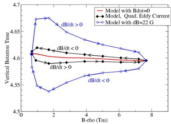
Figure 5: Results for  $\dot{B} = 8T/s$  of 2 different simulations.
