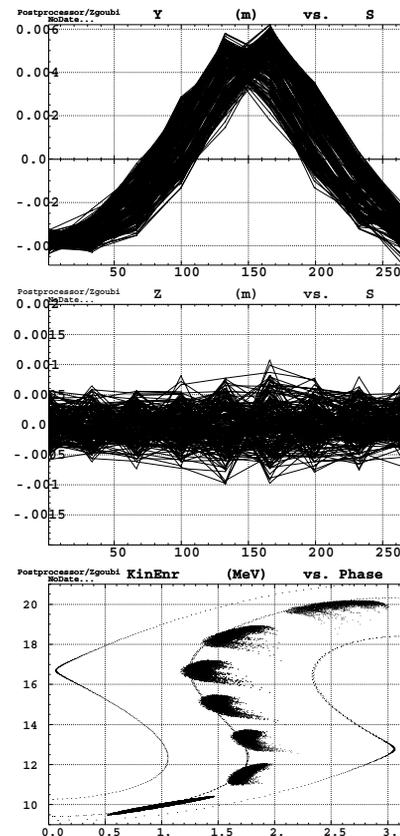
Figure 7: From top to bottom : (i) x-s and (ii) z-s during acceleration/deceleration (i.e., a full longitudinal period), observed along the ring at the location of the 14 cavities, (iii) longitudinal motion ; the plot also shows 2 trajectories close to the separatrix, and a third, central one.
