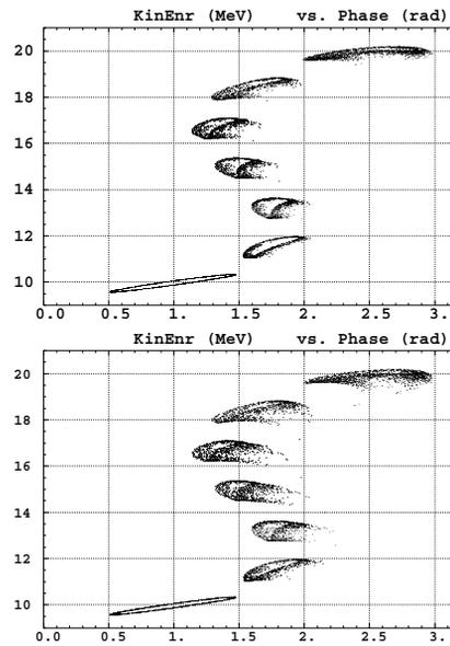
Figure 6: The sensible effect of launching a bunch with non-zero transverse size. Left :  $\beta\gamma\epsilon_x/\pi \approx 1.4$  mm, right :  $\beta\gamma\epsilon_x/\pi \approx 2.8$  mm.  $\epsilon_z = 0$  in both cases.
