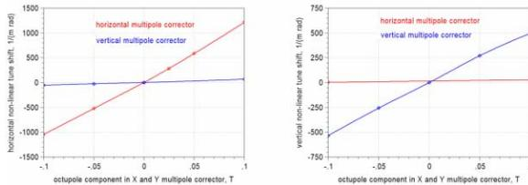
Figure 4: The non-linear tune shift versus the octupole components in multipole horizontal  $b_{oct}^{hor}$  and vertical  $b_{oct}^{ver}$  corrector.
