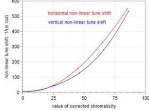
Figure 2: The horizontal and vertical non-linear tune shift versus the required corrected chromaticity  $\Delta \zeta_{cor}^2$ .
