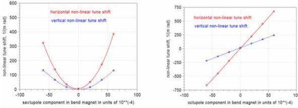
Figure 3: The non-linear tune shift vs the sextupole  $\Delta b_{sext\_mag} / B_0$  and octupole  $\Delta b_{oct\_mag} / B_0$  components in bend magnet.
