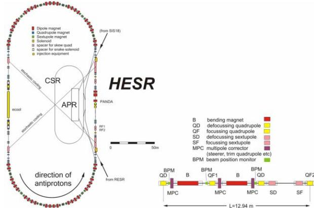
Figure1: Schematic layout of the HESR lattice and one half super-period.
