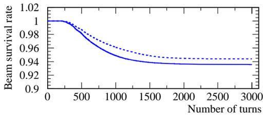
Figure 2: Beam survival as a function of turn number estimated for the bare working tune of (6.72, 6.35) without any resonance correction, in which the solid line shows the result from a simulation including all the intrinsic nonlinear fields listed in Table 1, while the dotted line is that including only the chromatic correction sextupole fields.
