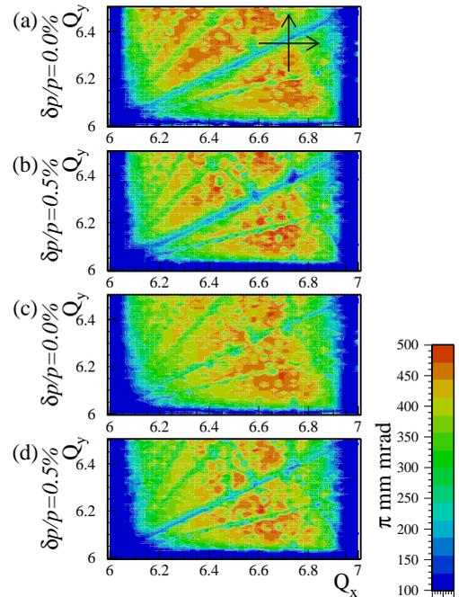
Figure 1: Dynamic acceptance maps as a function of  $Q_x$  and  $Q_y$  estimated for on- and off-momentum particles of  $\delta p/p = 0$  and 0.5% in the nominal operating region. The upper (a) and (b) show those before the correction of  $Q_x - 2Q_y = -6$ , while the lower (c) and (d) are after that.
