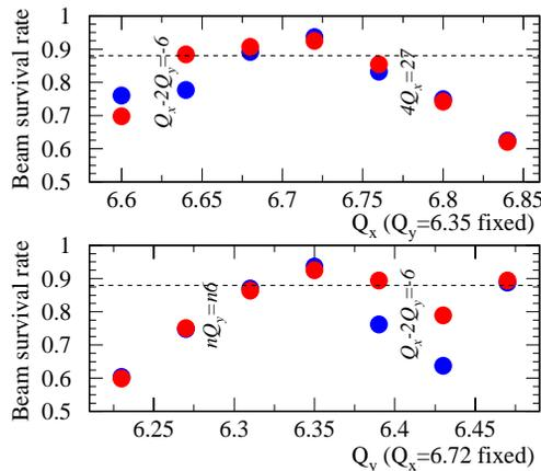
Figure 3: Beam survival rate at 3000 turns as a function of the working tune along the scanning lines shown in Fig 1-(a), in which the blue and red circles correspond to those without and with the  $Q_x - 2Q_y = -6$  resonance correction, and the dotted line shows the threshold corresponding to the limit of beam losses at the collimator (4 kW).
