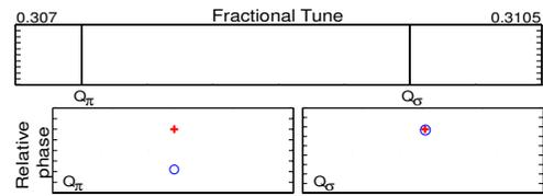
Figure 1: Eigenfrequencies and eigenvectors of a system of two bunches colliding head-on in one IP. The in and out of phase components are clearly visible for the two beams (crosses indicate beam one while circles beam two).
