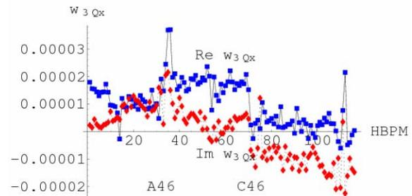
Figure 3: Generating function  $w_{3Q_x} = w_{3000}^{(meas)} \exp(3iQ_x\theta)$ . Jump associated with strong feeddown sextupoles at A46 and C46 can be clearly seen.
