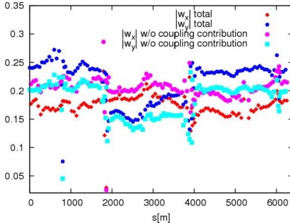
Figure 2: Functions  $w_{x,y}$  vs distance from F18 for Tevatron collision optics with tunes close to half-integer values: red and blue - as directly determined from data, magenta and cyan - with coupling contribution subtracted.
