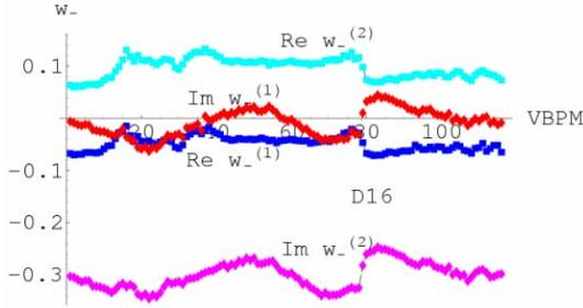
Figure 1: Real and imaginary parts of the difference resonance generating function seen at the Tevatron vertical BPMs starting from F18: blue and red – far from the resonance, cyan and magenta – close to it.
