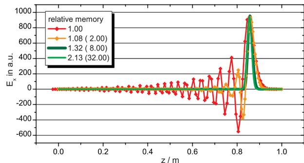
Figure 3: With increasing refinement level the resolution increases and the numerical phase velocity approaches the speed of light in vacuum (top). Gaussian packet for the refinement levels 0, 1, 3 and 5. In the legend the memory needed for the time-adaptive mesh approach and a static grid of equal resolution (in brackets) are given (bottom).
