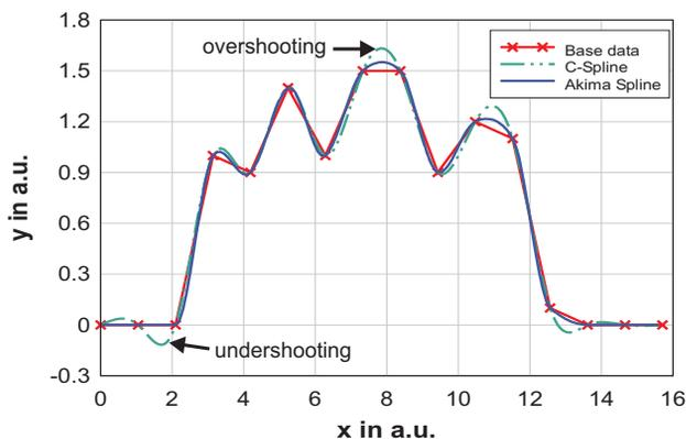
Figure 2: Comparison of a C-Spline and an Akima-Spline. The Akima-Spline shows less overshooting and because of the slope limiting it is smoothed out to a constant at both ends of the curve.
