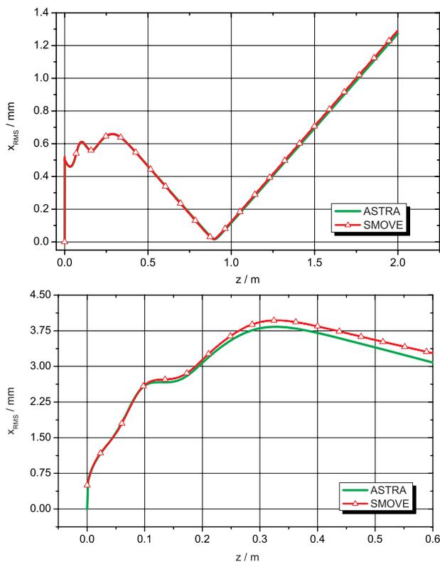
Figure 4:  $x_{RMS}$ -size calculated by SMOVE and ASTRA in tracking mode (top) and in self-consistent mode (bottom). The simulation of longer distances is easily possible without any memory problems.
