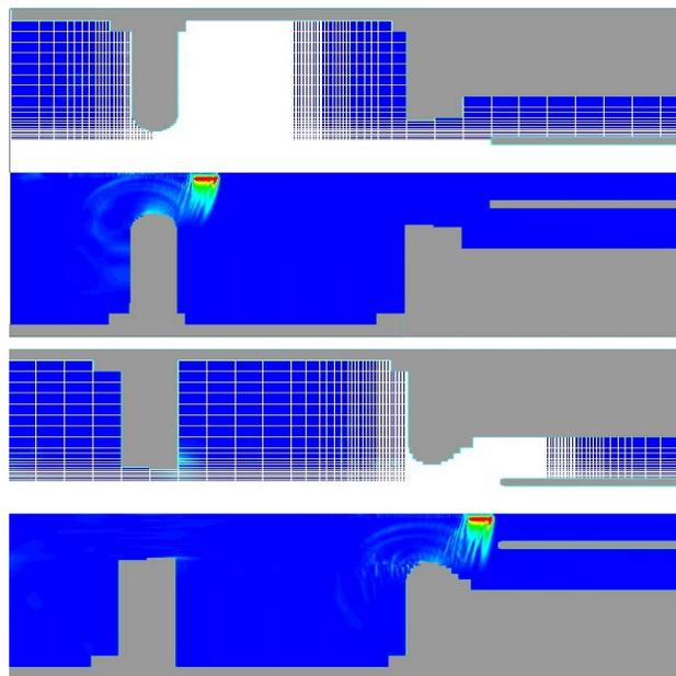
Figure 1: Computational grid and space charge fields for the PITZ gun. The discrete material representation changes with time according to the local resolution of the dynamic grid. This can be seen by comparing the metallic contours in both snapshots.
