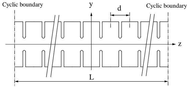
Figure 1: A rotationally-symmetric periodic structure.
