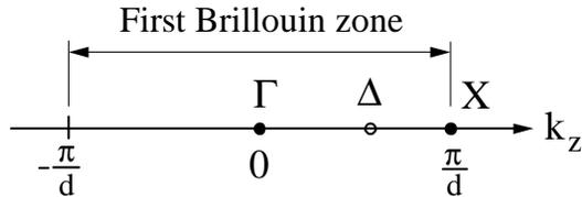
Figure 2: Brillouin zone for the one-dimensional periodic structure.
