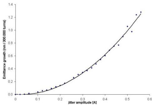
Figure 7: The simulated emittance growth due to a turn-to-turn current-amplitude jitter for a wire length of 1m and a quadratic fit ( $4 \times 10^{-9} I^2$ ).
