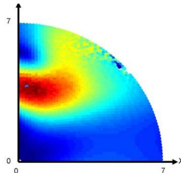
Figure 9: The Liapouov-exponent after 300.000 turns for a single LR-BB interaction at  $3.5\sigma$  in RHIC (blue: low, red: high).
