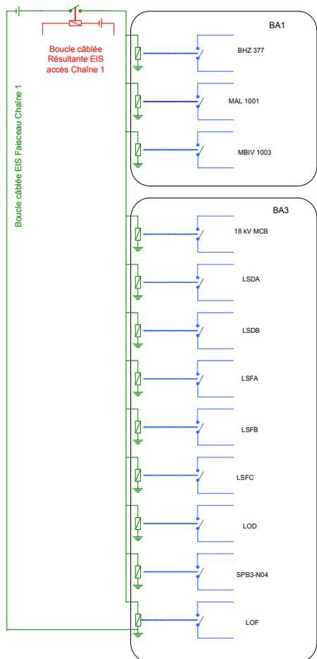
Figure 5: Functional schema of the cabled loop EIS-f of the safety chain 1.
