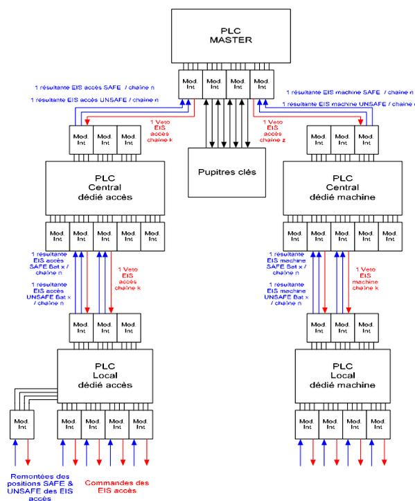
Figure 2: The SPS access system architecture
