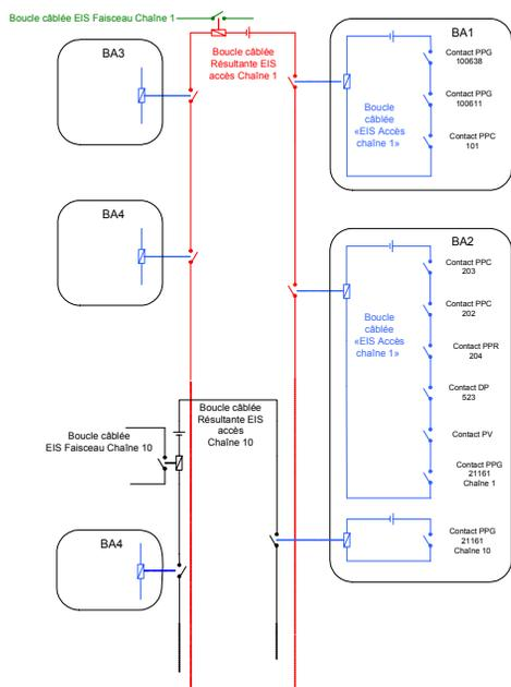
Figure 4: Functional schema of the cabled loop EIS-a. For the simplicity of illustration, only the EIS-a of the access point in BA1 and BA2 have been represented on this picture.
