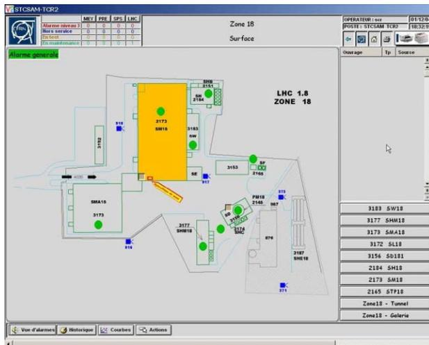
Figure 2: Alarm synoptic view on the CSAM HCI.
