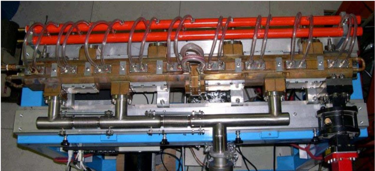
Figure 2: First SCDTL module during the RF tests in Frascati
