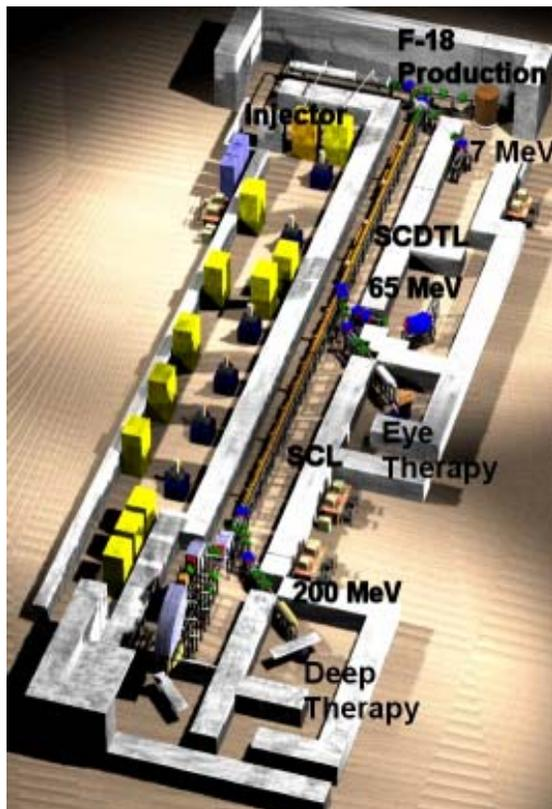
Figure 1: 3D drawing of the TOP linac
