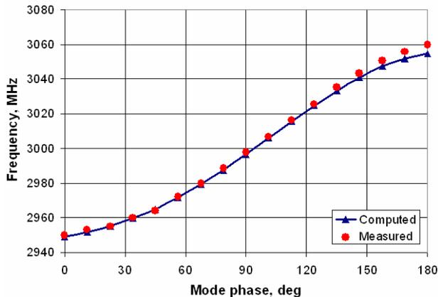
Figure 4: measured and computed mode frequencies
