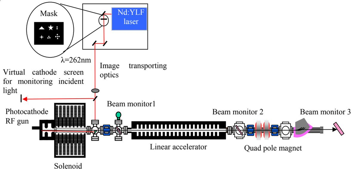
Fig. 2 The laser photo cathode electron linear accelerator with the optical processing incident optical system (photo-masks and image transport optics) and the electron beam monitor (desmarquest plate and CCD camera)
