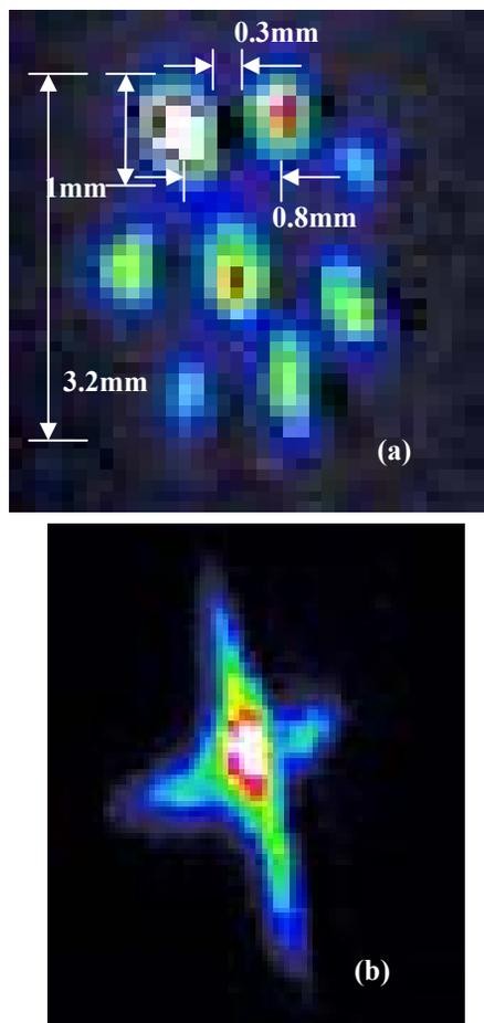
Fig.4 Spatially resolution of (a) the multi spots electron beam and (b) the cross shape electron beam
