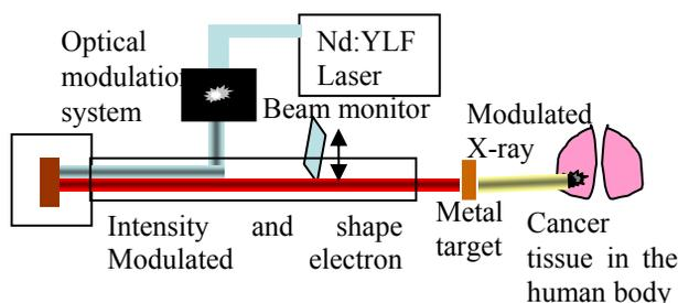
Fig.1 Concept figure of the Intensity modulated radiation therapy by the photo-cathode electron accelerator
