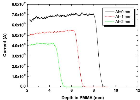
Figure 6: Dependence of depth-dose distribution on the incident beam energy.
