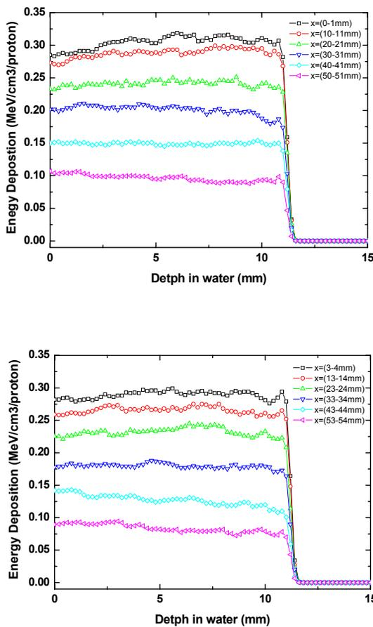
Figure 3: Depth-dose distributions simulated by MCNPX for the optimized ridge shape.
