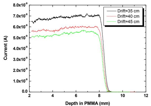
Figure 5: Dependence of depth-dose distribution on the drift distance.
