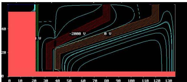
Figure 3: Trajectory of ion beam using igun code.
