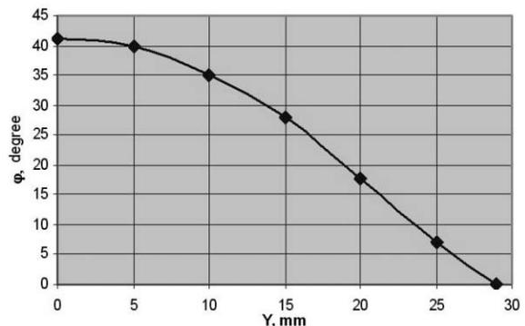
Figure 5: The phase shift depending on Teflon plate position for one wave pass through the phaseshifter.
