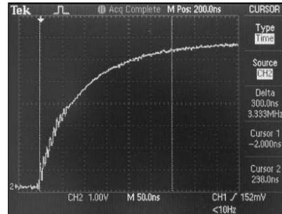
Figure 8: Measured rise time in one module model.
