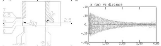
Figure 1: Calculated injector geometry (mm) and beam trajectory (cm).
