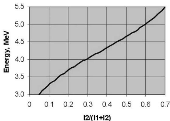
Figure 3: Calibration chart of energy measurement unit.
