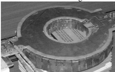
Figure 7: The model of the pulse transformer module.
