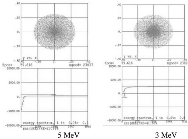
Figure 2: beam cross-section distribution and energy spectrum.
