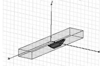
Figure 4: Teflon plate phaseshifter.
