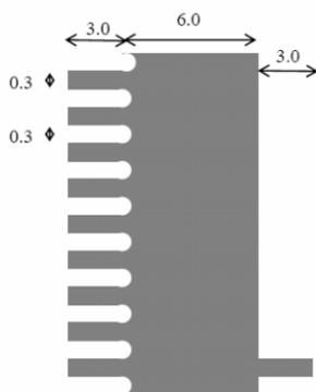
Figure 3: Section of the readout vane.
