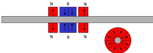
Figure 2: The shuttle magnet assembly.
