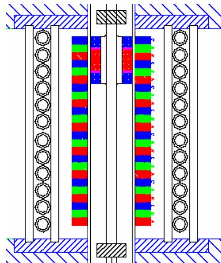
Figure 1: The stator, also showing the shuttle magnets.
