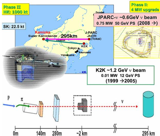
Figure 3: Top: Overview of the J-Parc to SuperKamiokande long baseline experiment foreseen from 2009. Bottom: Schematic description of the detectors along the T2K beam line.
