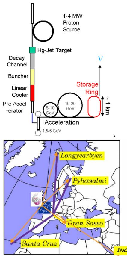
Figure 5 Top: the neutrino factory accelerator complex; bottom: possible beam lines in Europe.
