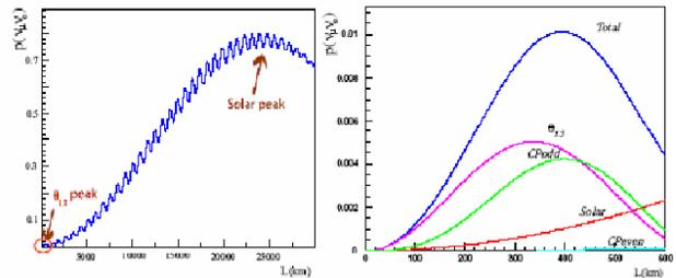
Figure 2: Description of neutrino oscillations for 1 GeV neutrinos as a function of distance to the source. The oscillation parameters are  $\sin^2 2\theta_{13} = 0.01$ ,  $\delta = 0$  for the left plot,  $\delta = -\pi/2$  for the one on the right, which shows the CP violating terms at the first oscillation.
