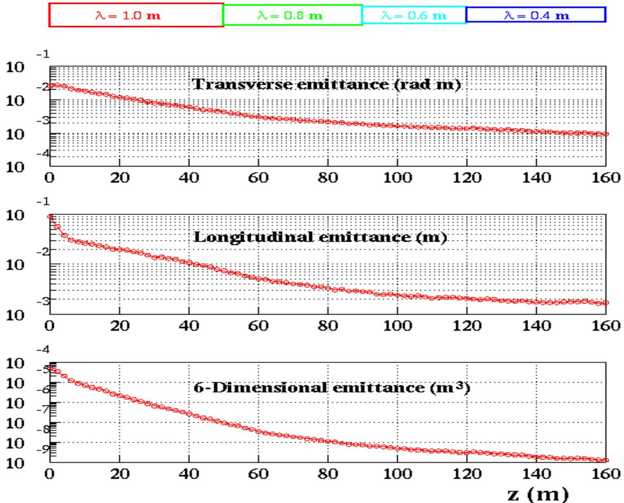
Figure 2: Emittance evolution of a muon beam in 4 sequential HCC segments. The cooling factor is 50,000 in a total channel length of 160 meters. The final emittances will be improved with a better simulation model.
