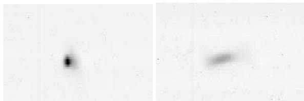
Figure 9: Unprocessed bunch images. Left: RFD switched off. Right: RFD on, at zero-crossing phase.
