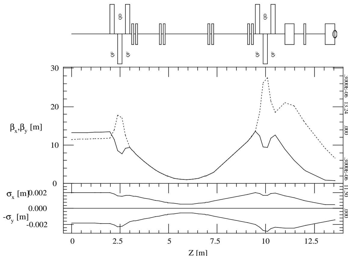
Figure 5: Drive-beam optics
