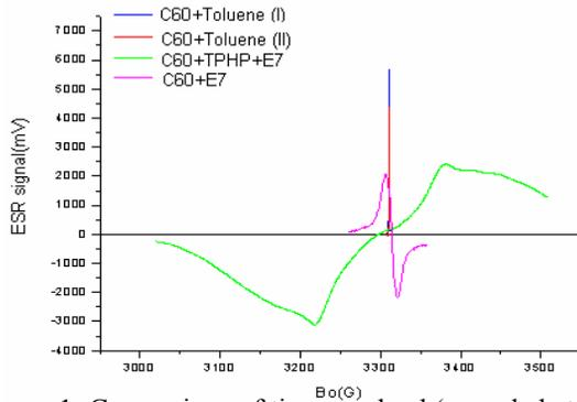
Figure 1: Comparison of time resolved (recorded at a fixed delay with respect to the laser pulse) EPR spectra for some of the test samples. Positive signal corresponds to absorption, negative to emission.  $1G = 2.8 \text{ MHz}$ ; the position of the reference absorption peaks corresponds to  $9.27 \text{ GHz}$  [8].
