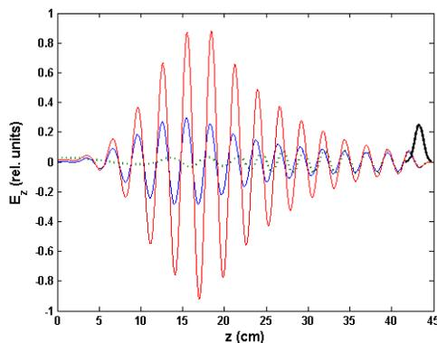
Figure 3: Arrakis simulation of the longitudinal wakefield of a beam in an X-Band dielectric structure. Black: beam pulse; Green: wake from passive dielectric; Red: active structure; Blue: active structure with lossy dielectric.
