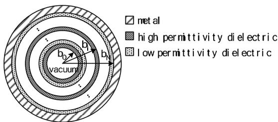
Figure 1: Cross-section of the multilayered dielectric-loaded accelerating (DLA) structure. The structure is a cylindrical waveguide which consists of a vacuum core with radius  $b_0$  surrounded alternating high and low permittivity dielectric tubes with outer radius  $b_1$ . A conducting jacket encloses the structure.
