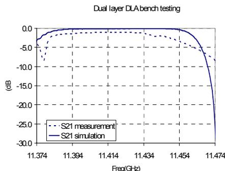
Figure 2: Comparison of the results of the bench testing and the rf transmission simulation of the structure with a single section of double layer ceramic tube.
