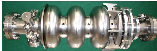
Figure 2: Photograph of the 3 1/2 cell Nb cavity.
