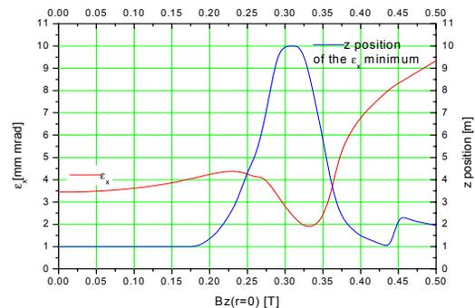
Figure 6: Transverse emittance in dependence on the magnetic axis field.
