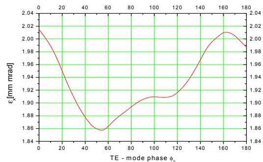
Figure 5: Transverse emittance in dependence on the TE – Mode.
