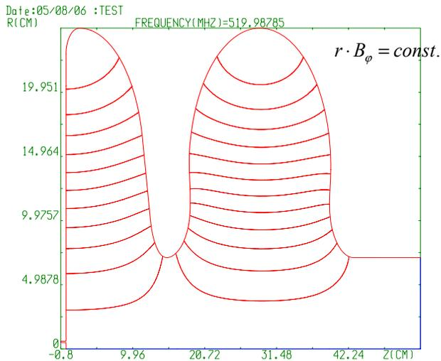
Figure 1: Cavity shape and field distribution of the TM mode.
