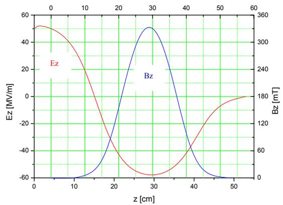
Figure 3: Axis fields of the cavity.
