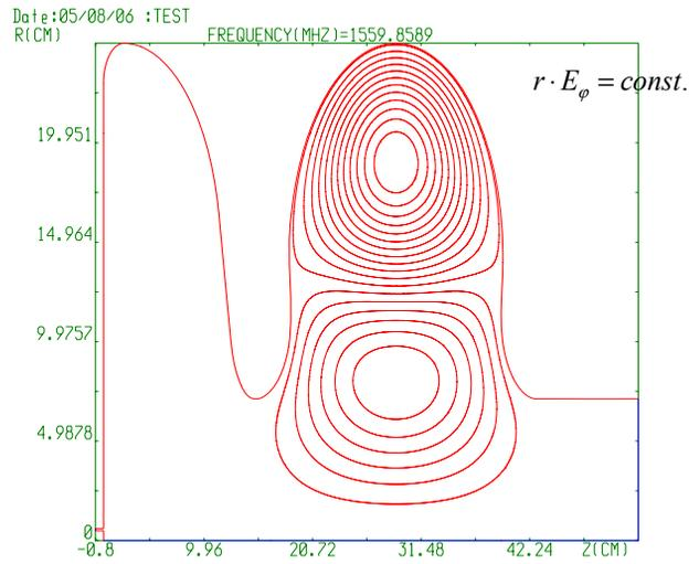
Figure 2: Cavity shape and field distribution of the TM mode.
