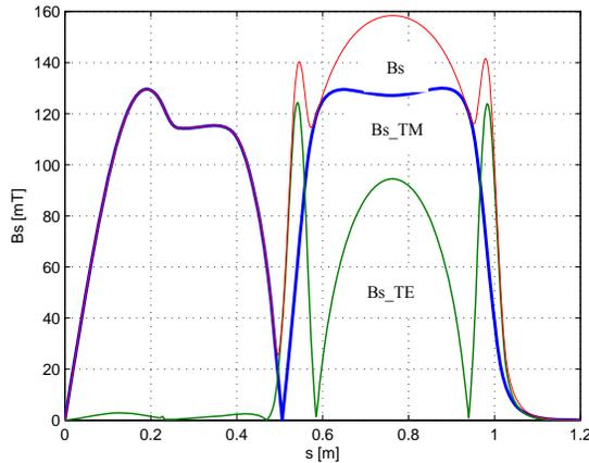
Figure 4: Magnetic surface fields in dependence on the surface coordinate  $s$ ,  $B_s = \sqrt{(B_s\_TM)^2 + (B_s\_TE)^2}$ .
