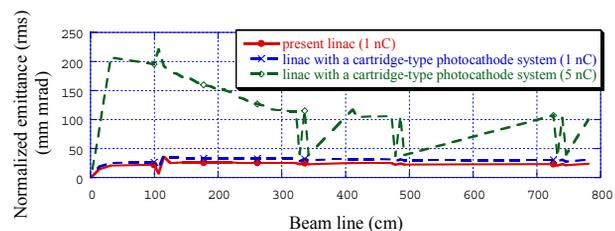
Fig.6 PARMELA simulation of the emittance (rms) along the linac. The emittance at the end of the linac: 24 mm mrad in present linac (1 nC), 32 mm mrad in linac with a cartridge-type photocathode system (1 nC), 100 mm mrad in linac with a cartridge-type photocathode system (5 nC)
