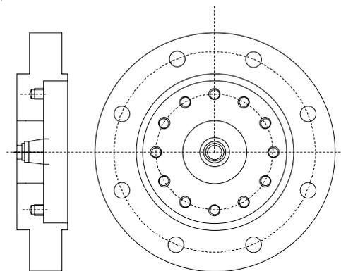
Fig. 3 Design drawing of the back plate with a hole
