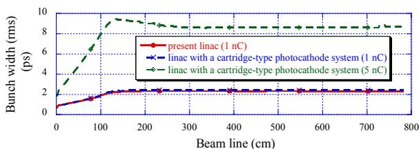
Fig.5 PARMELA simulation of the bunch width (rms) along the linac. The bunch width at the end of the linac: 2.3 ps in present linac (1 nC), 2.4 ps in linac with a cartridge-type photocathode system (1 nC), 8.7 ps in linac with a cartridge-type photocathode system (5 nC)
