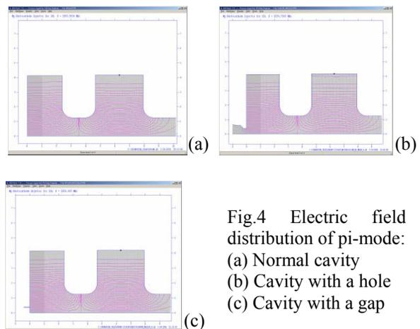
Fig.4 Electric field distribution of pi-mode:
