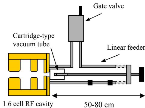
Fig. 1 Schematic view of RF cavity with a cartridge-type photocathode system
