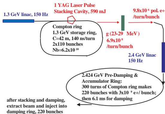
Figure 1: Schematic view of CLIC Compton source.
