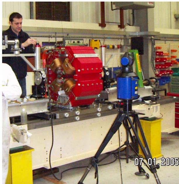
Fig 1 Surveying the rotating coil bench, mounted on a Diamond girder.
