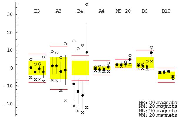
Fig 2 Harmonic Results for 20 worst magnets of each type, as built. See fig 4 for key.
