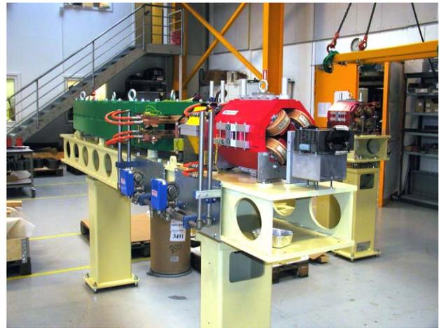
Figure 9: Girder Assembled with Dipole, Sextupole and Quadrupole magnets.
