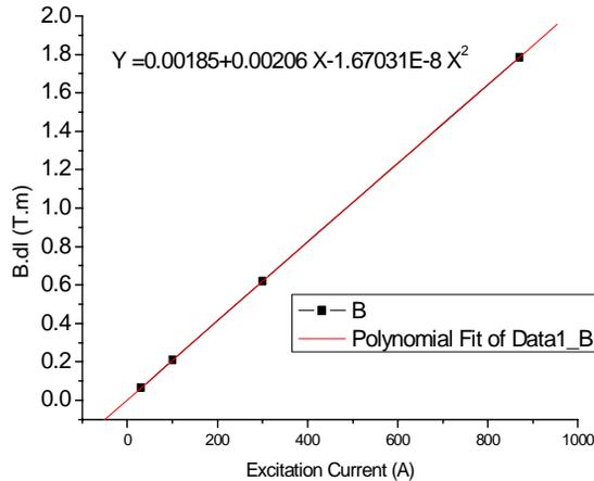
Figure 4: Dipole Magnet Excitation Curve
