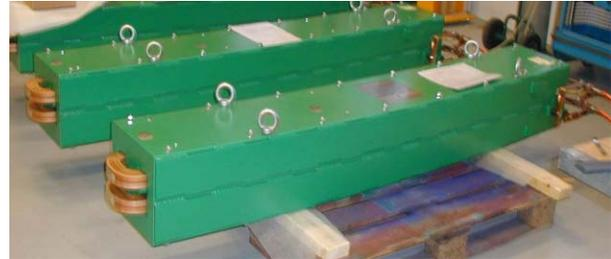
Figure 1: Dipole magnets
