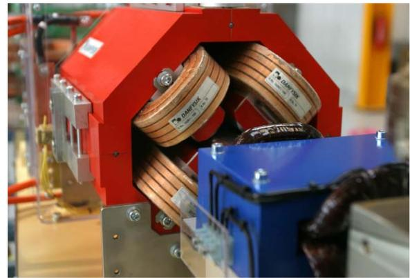
Figure 5: Quadrupole magnet
