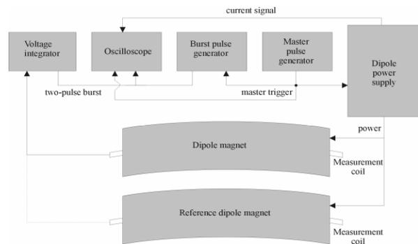
Figure 2: Integrated field measurement setup
