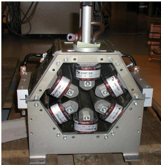
Figure 8: Prototype Sextupole Magnet
