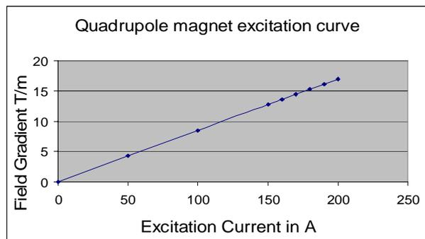
Figure 7: Excitation Curve for Quadrupole Magnets
